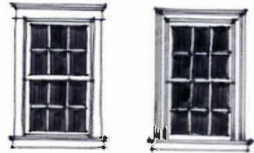
SIMPLE HEAD & JAMB TRIMS WITH SIDING/ MORE DETAILED WITH STUCCO
