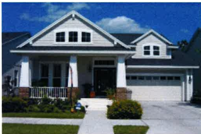
BATTERED COLUMNS / MULTIPLE ROOF PLANES
